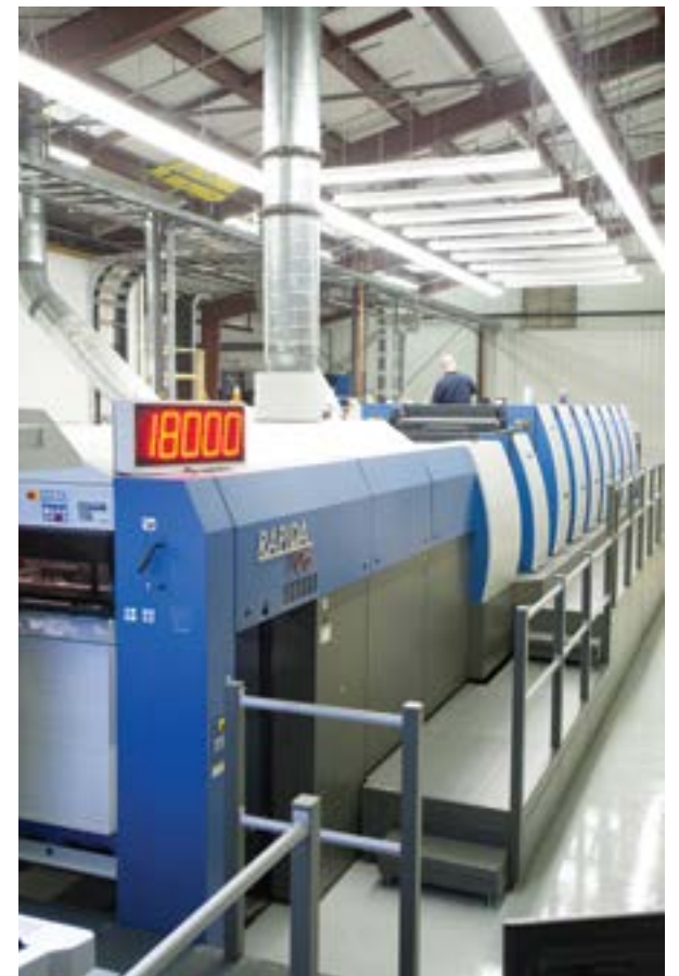
With maximum throughput of 18,000 sheets per hour, the KBA Rapida 106 seven-color printing press with a coater and UV dryer was custom-built to Ingersoll Paper Box's exact specifications.
