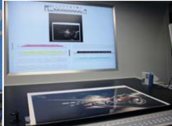
The KBA live-image QualiTronic ColorControl wall screen provides the Rapida 106 press operators with a visual inline color measuring system to ensure print integrity is maintained throughout the run. Photos by Andrew Joseph.
