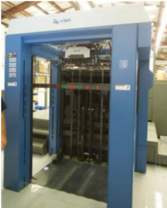
Ingersoll added the optional automatic pallet changer with safety light curtains for the feeder section of the Rapida 106 printing press.
