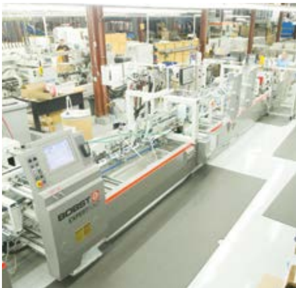
The EXPERTFOLD 110 A-2 high-speed folder-gluer manufactured by BOBST utilizes the unique AccuBraille application system to apply the Braille language codes onto the paperboard packaging.
