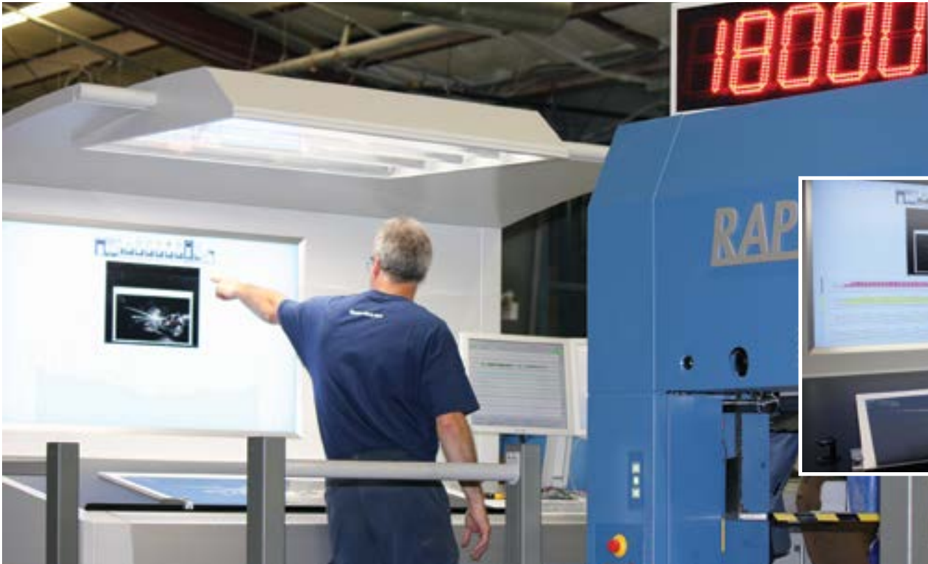
The KBA live-image QualiTronic ColorControl wall screen provides the Rapida 106 press operators with a visual inline color measuring system to ensure print integrity is maintained throughout the run. Photos by Andrew Joseph.
