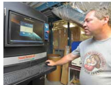
An employee dispenses printing press ink with the easy-to-use, Mx12 ink formulation and dispensing system supplied by Sun Chemical.
