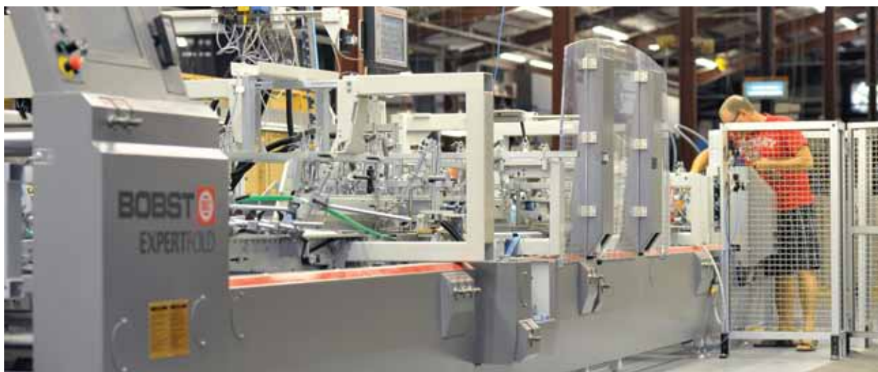
An Ingersoll Paper Box employee preforms a routine maintenance check on the company's new Bobst Expertfold 110 A-2 folder-gluer, said to be the only one of its kind in North America to also run a Braille application system.
