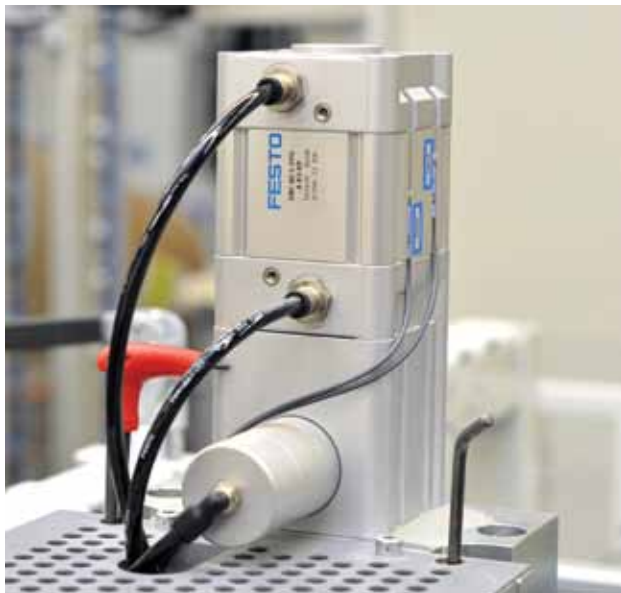
Festo pneumatics are utilized to press paperboard packaging up against the AccuBraille application system.
