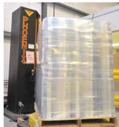
A Phoenix Innotech stretchwrapper stabilizes a load of die-cut paperboard packaging.
