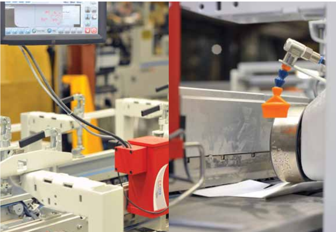
A Valco Melton Captor vision inspection system (left) added to Ingersoll Paper Box's new Bobst Expertfold 110 A-2 folder-gluer checks the veracity of its Bobst AccuBraille application system (right) that embosses Braille language data onto the pharmaceutical packaging.
