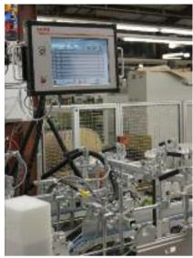
technology and custom lighting, it examines each Braille embossed carton at full production speed, checking the depth and accuracy of each dot.
